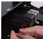
安装Y轴限位开关保护罩 Install the Y-axis limit switch protective cover
