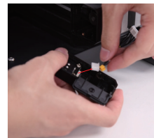
拔出Y轴限位开关线 Pull out the Y-axis limit switch cable
